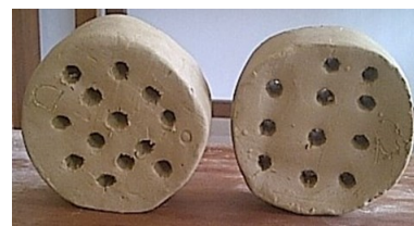
Plate 2: Green bodies after formation of honeycomb structure
