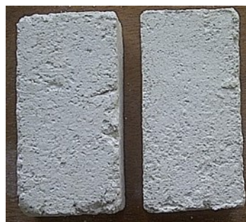
Plate 1: Green bodies after firing with PHDPE as pore former
